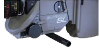
Finding the camera's fore-aft c.g.
