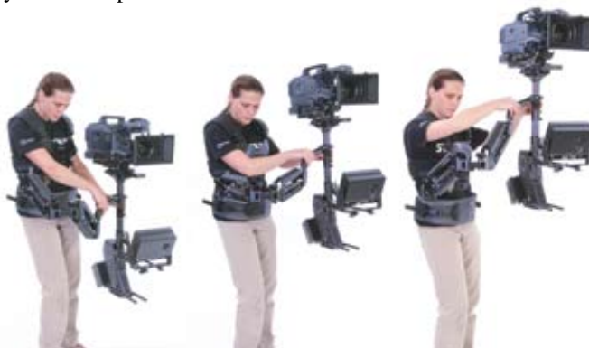
Boom the arm up and down, watching to see if the upper arm follows the forearm.
