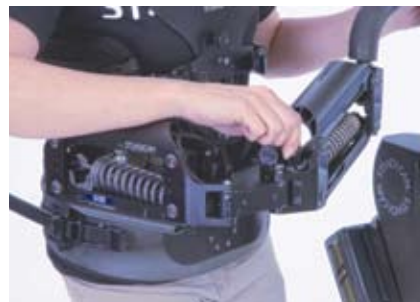
Adjusting the forearm section. The arm must be angled slightly up for the adjustment screw to turn.
