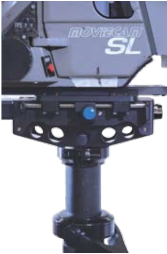
Camera's fore-aft c.g. .75" behind center post.
