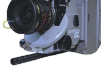
Finding the camera's side to side c.g.
