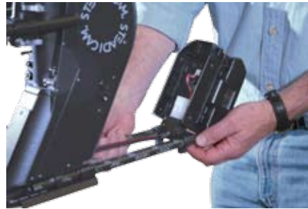
Camera c.g. is .75 inch behind the centerline of the post. Pull out the battery.
