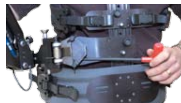
Use a 1/4” allen to adjust the “side-to-side” screws. When wearing the rig, be sure to hold the centerpost in line with the “in-out” thumbscrews. This will take the loading off the side-to-side screws.
