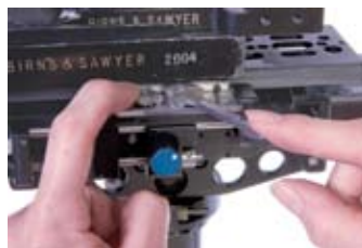
The button must be depressed to open dovetail locking lever fully.
