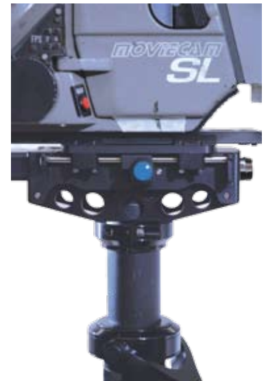
Camera c.g. is .75 inch behind the centerline of the post. Pull out the battery.
