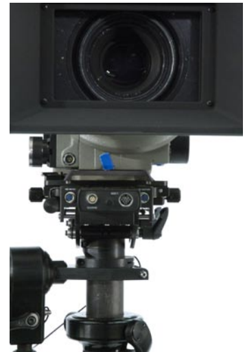
Camera c.g. centered over post – side to side.
