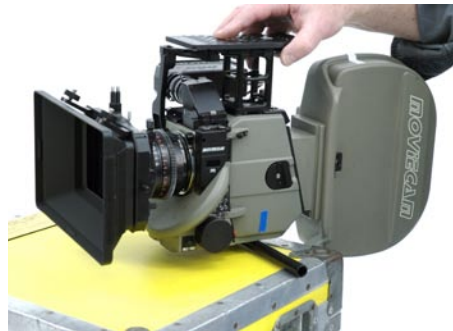
Finding the camera's fore-aft center of gravity.
