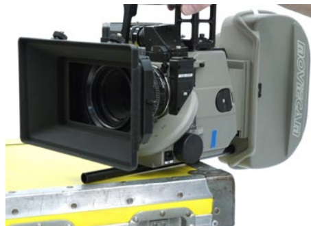
Finding the camera's side to side center of gravity.
