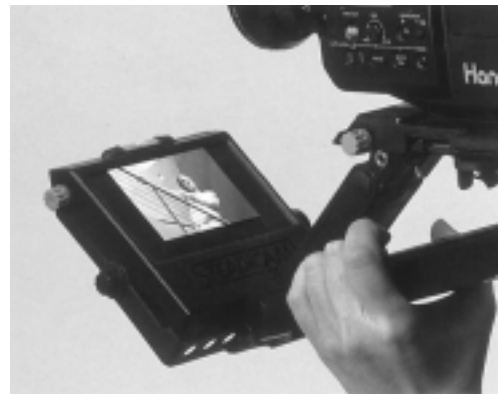
A special optical filter reduces glare on the monitor to less than .4%, even in direct sunlight.
